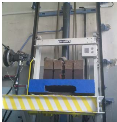
fig. 5 Hydraulic elevator test bench with energy regeneration system [7]
